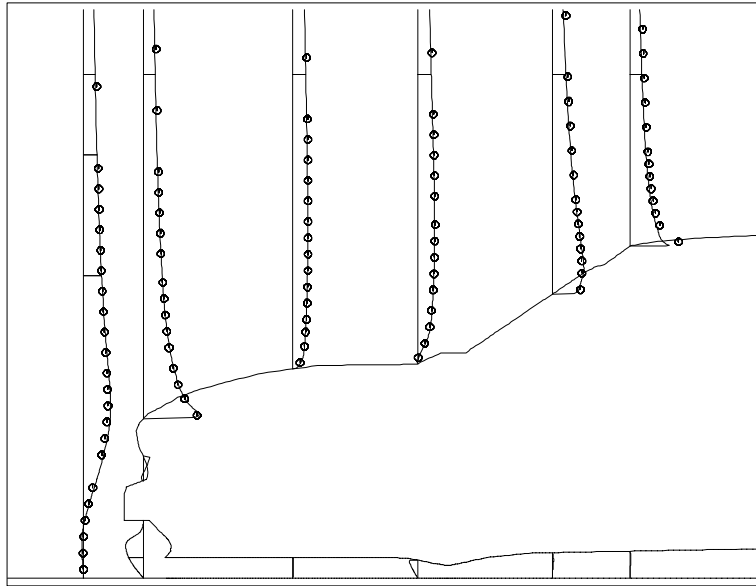
Figure 11. Comparison of numerical (lines) and experimental (circles) profiles of velocity component V .
